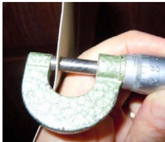
Fig 9. Measuring the Thickness of a Sheet of Parchment with a Micrometer.
